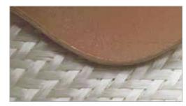
Edging Synthex is a snap using traditional techniques and applying Fabtech EasyEdge Composite Sealer.
